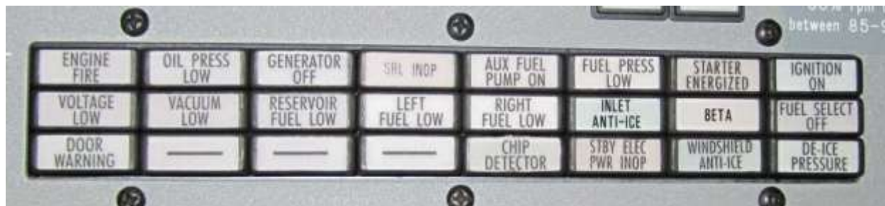
Figure 7-1, Modified Annunciator Panel PRE Supervan Systems SB 208-7
