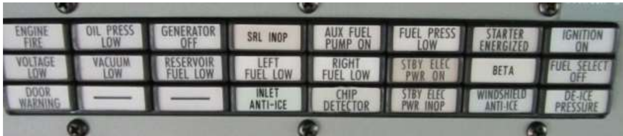
Figure 7-1A, Modified Annunciator Panel POST Supervan Systems SB 208-7
